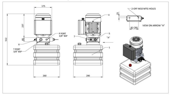
Motor: 1 PH 0.75Kw 1450 rpm Helical Gear Pump: 5.00 cc/rev
